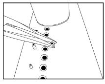
**2.** Insert 3/16" x 1/2" pin as shown. Hold pin with needle nose pliers. Gently hammer pin until .100" remains above the tool surface. Repeat for all pins this size.
