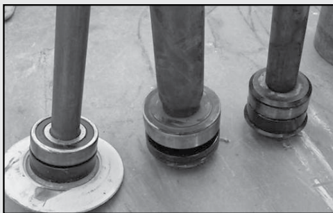
The CoreTech Roller on the left shows no signs of internal corrosion, while the two steel rollers on the right showed clear signs of corrosion on the shaft, as well as around the bearing.
