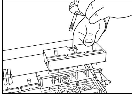
2. Lift cam lever and remove cam lever and guide block over the damaged anvil.
