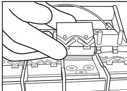
8. Remove damaged anvil from the tool.
