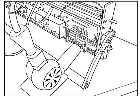
6. Put on heat resistant gloves. Use a 1500W heat gun on high and heat the anvil for approximately 10 minutes. (Caution - Please read all manufacturer instructions on proper use of the heat gun). This will loosen the Loctite. Allow time for plate and screws to cool.
