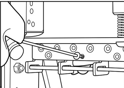
7. Using enclosed Allen wrench, turn three screws counterclockwise.
