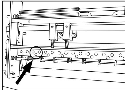
5. Turn tool on its side and identify the three screws that secure the anvil to be replaced.
