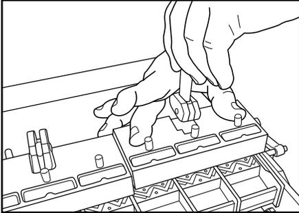
1. Release cam lever, press down block and turn cam lever counterclockwise.
