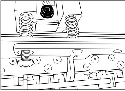
**10. For tools with anti-lifting mechanism only:** Replace the anti-lifting mechanisms from the top of the tool. Next, apply Loctite to the end of each screw (total of 4) and slowly thread until they have engaged in the tool. Replace the (4) springs and continue to tighten the screws (screws go through the center of each spring) until fully seated.
