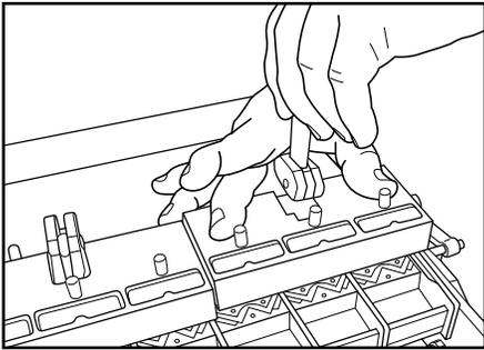
**13.** Replace guide block and cam lever. Tighten cam lever. Do not use tool for 24 hours to allow Loctite to dry.
