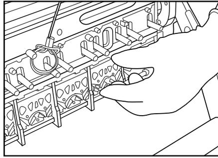
**11.** Hold anvil plate, line up screws, and tighten all three screws.
