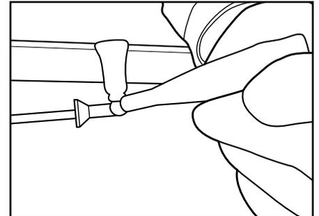
9. Open enclosed Loctite tube and apply Loctite to the three anvil screws included in this package.
