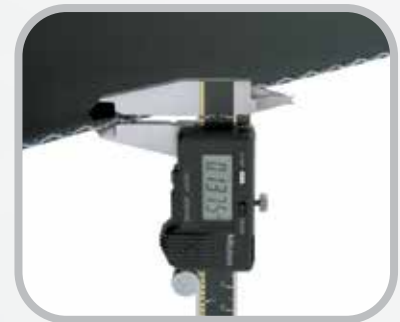
Measure belt thickness.
