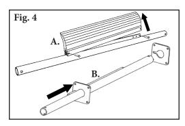
**4. Install the pole.** Remove both blade pins and blade from the pole and insert the pole in through the mounting plates (Fig. 4).
