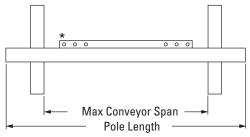
\*Each pole size can be used with a blade size either belt width minus 50mm, belt width minus 200mm, or belt width minus 350mm.
