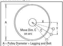
C = Critical Spec to move location if necessary
