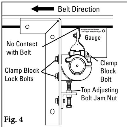
4. **Set the tip angle.** With angle setup gauge provided, rotate the tips to the preset angle (Fig. 4) and lock the pole in place by tightening the clamp block bolts equally. **NOTE:** Make sure there is NO tip-to-belt contact while making this alignment. If contact occurs, lower the pole by loosening the clamp block lock bolts and raising the top adjusting bolt jam nut (Fig. 4). When tips are lowered and not touching the belt, repeat this step.
