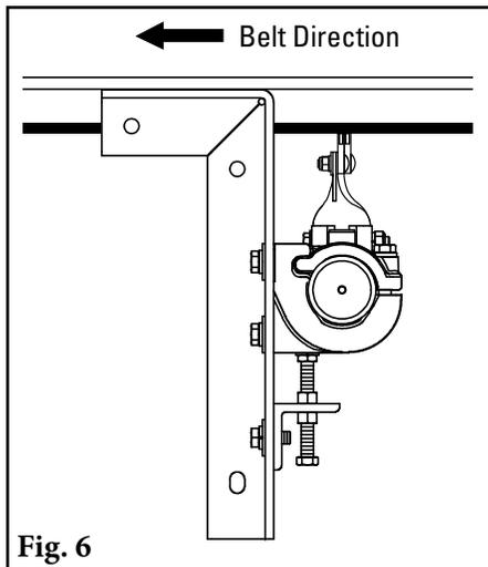
6. **Check the tip tension.** Pull back on the outside tip until the belt-to-tip contact is broken and release. The total blade thickness of the adjacent tip must be visible (Fig. 6). Add or reduce tension by 1/4 turn (see Step 5) until full thickness of the adjacent tip is visible.
