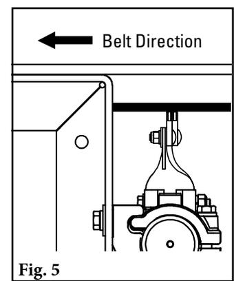
**Test run cleaner and inspect operation.** If vibration occurs, increase tip tension by making 1/4-turn adjustments.
