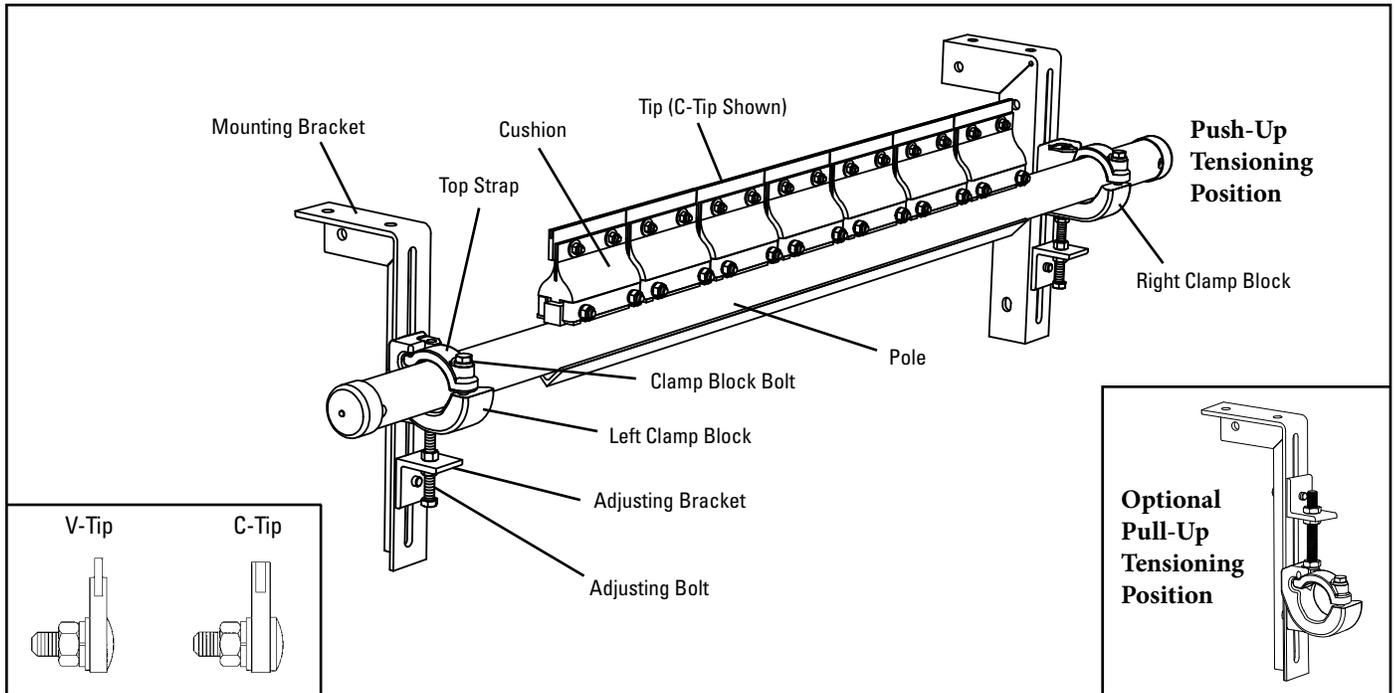
***Physically lock out and tag the conveyor at the power source before you begin cleaner installation.***
