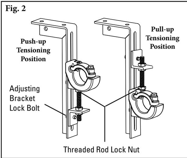
2. **Choose the tensioner position.** The tensioner is shipped mounted in the push-up position. Depending upon the space constraints of the installation, the tensioner can be optionally mounted in a pull-up position. To do this, loosen the threaded rod lock nut, unscrew the threaded rod and remove adjusting bracket lock bolt. Then move the adjusting bracket and threaded rod to the top of the clamp blocks (Fig. 2) and tighten threaded rod lock nut.
