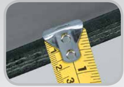
Measure belt thickness
