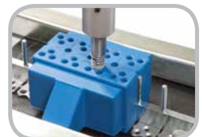
Air Powered Rivet Driver Installation
