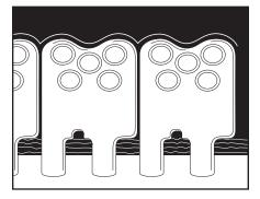
11. Remove guide block(s) and make sure rivets are set completely. Complete belt end by moving the block across the width of the belt and continue driving rivets.
