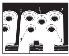
**10.** Drive rivets into the center hole of both end plates. This will anchor fastener strip in position. Continue to drive all remaining rivets into holes in the sequence shown above.
