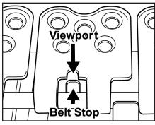
**5.** Center belt in fastener strip. Look through viewports, belt end should be tight against belt stops. Tighten hold down bar to secure belt.
