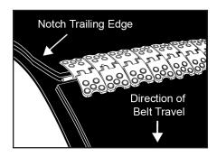
**13.** Repeat steps 1-12 on other belt end. Bring belt ends together and insert hinge pin. Notch trailing edge of belt only. Splice is complete.
