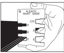
**2.** Measure belt thickness from cut edge using gauge or tape measure. Select correct size SR rivets for your belt thickness.
