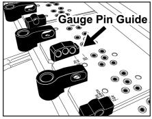
**3.** Place tool on wooden board, width of the conveyor framework, for support. Lift and turn gauge pin guide to correct fastener size.
