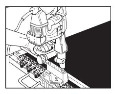
9. Insert the punch directly into the SR700 Guide Block. Keeping the tool perpendicular to the base, pull the trigger to fire the driver. Push down on the driver slightly and maintain force on the driver until you feel the rivet set. This should take approximately 1 to 2 seconds per rivet depending on the length of the rivet and the type of belt.
