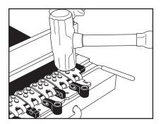
**12.** Remove guide blocks. Using a 4 lb (1.8 kg) hammer, set all rivets. The belt should pucker around the edges of the fasteners.
