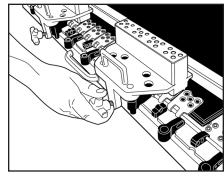
**6.** Set all fastener top plates with hammer blows. Place SR700 guide blocks at each end of the fastener strip and tighten clamping screws. Spray guide block with SL5 Silicone.
