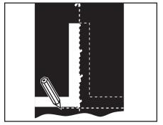
1. Square belt using centerline method. Cut belt at least 4"(100 mm) behind old splice using a Flexco belt cutting tool. Skive belt when top cover permits.
