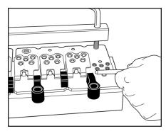
**4.** Center fastener strip on tool, Flexco stamp facing up. Holes on fasteners and anvil plate must line up. Insert gauge pin through guides and fastener loops.
