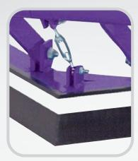
A corrosion-protected turnbuckle allows the blade to be fine-tuned to the belt at installation. This means the nose of the plough is accurately positioned so it will not dig into the belt and potentially cause damage to the belt or the plough. It also eliminates vibration that is typical with ploughs using chain links for adjustment.
