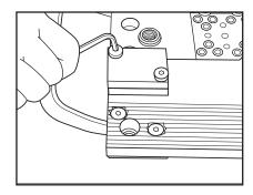
**5.** Place Screws into locator block. Use allen wrench to tighten screws.
