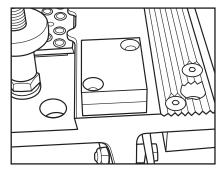
**3.** Place new locator block on top of existing locator block. Total height will be approximately 3/4" (19 mm). Align screw holes.
