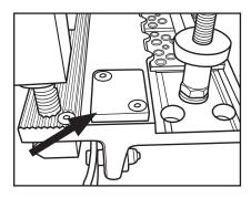
1. In order to retrofit a cambered clamp bar, you need two locator blocks stacked on top of each other. Check locator block at each end of the tool. If you already have two locator blocks – total height will be approximately 3/4" (19 mm) – stacked at each location, you do not need to continue. Tools shipped prior to 2010 have only one locator block.
