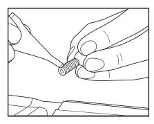
**4.** Apply loctite (included) to new locator block screws (included).
