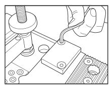
2. Loosen and remove locator block screws with the included 5/32" allen wrench. Discard screws.
