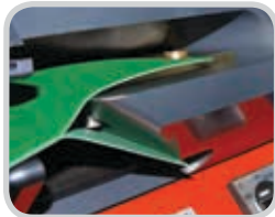
Accurate separation between belts, with cuts as thin as 0.014" (0.35 mm)
