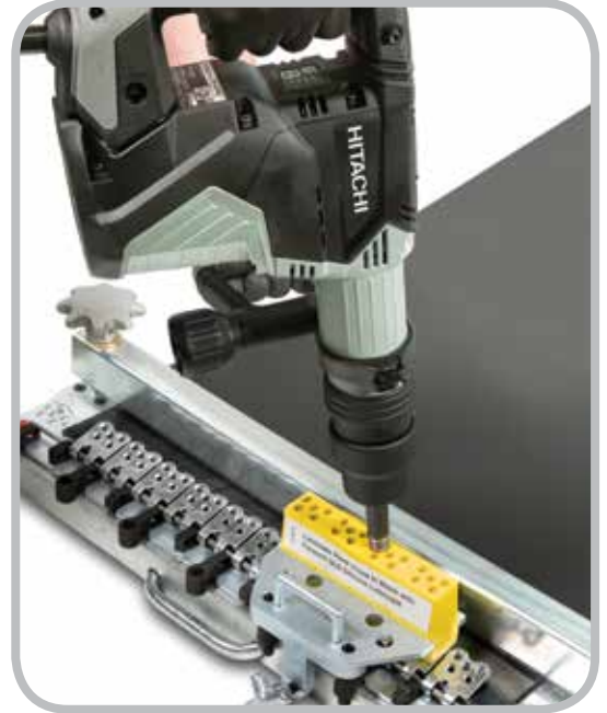
Electric Powered Rivet Driver Installation
