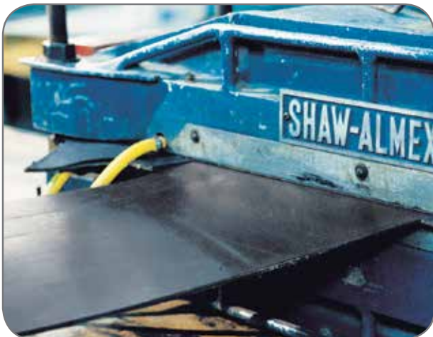
Hot vulcanized splices are cured in a vulcanizing press over time and under pressure.
