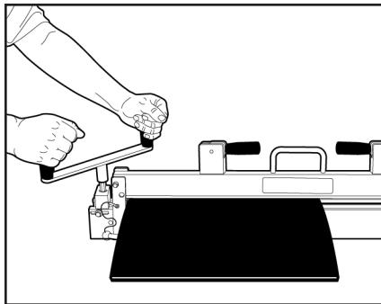
6. Fit wrench (E) on drive shaft (F). Turn wrench (E) clockwise/counterclockwise until blade completes cut and is secured in safety area.
