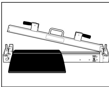
**3. Position belt against end of cutter, opposite blade. Align one edge of the clamp bar (A) with square mark.**
