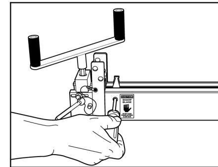
**Chain Tensioner:** Loosen bolts on slotted end with wrench (E). Adjust drive shaft (F) by hand to desired tension. Tighten bolts.
