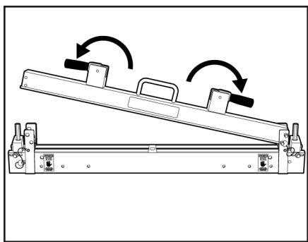
**2. Move blade to end of cutter. Unlock clamp bar handles (B). Remove lock pin (C). Lift clamp bar (A). Insert prop pin (D).**
