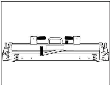
**To Store Wrench:** Raise clamp bar (A). Insert wrench (E) in hole. Close and lock clamp bar (A).
