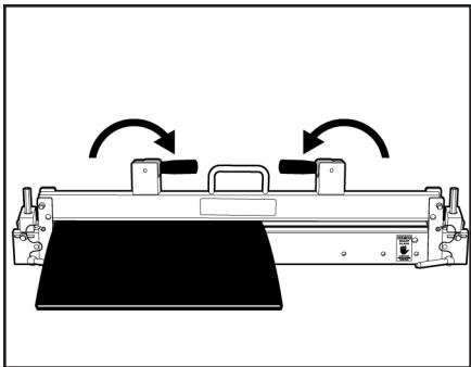
5. Remove prop pin (D). Lower clamp bar (A). Insert lock pin (C). Align square mark and lock clamp bar handles (B).
