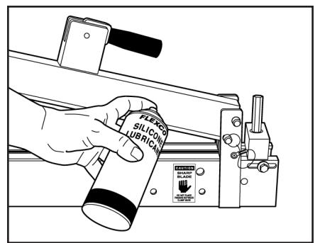
**4. To improve cutting and blade life, spray blade with Flexco® Silicone Lubricant.**
