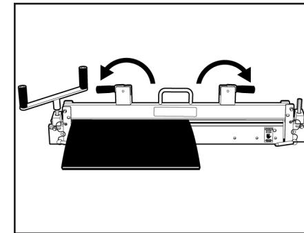
7. Unlock clamp bar handles (B) and remove belt.
