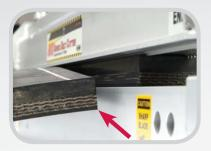
The single-sided clamp feature allows the cut belt to fall free on one side, eliminating the need for the blade to cut through two clamped surfaces, reducing operator effort.
