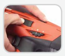
Easily adjust the Hilti DX 460-SR to the correct power setting for the rivet size and belt type for your installation.
