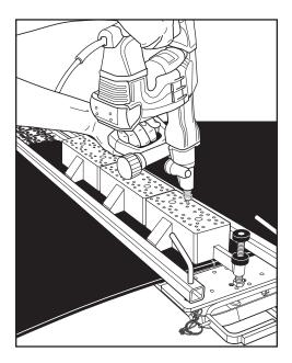
**15**. Adjust setting dial for rivet size – see chart below. Insert the punch directly into the BR500 Guide Block. Keeping the tool perpendicular to the base, pull the trigger to fire the driver. Push down on the driver slightly and maintain force on the driver until you feel the rivet set. This should take approximately 1 to 2 seconds per rivet depending on the length of the rivet and the type of belt.
