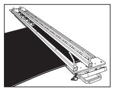
**10**. Place belt against clamp bar (B). Center belt over bottom plates. Clamp belt to tool with the other clamp bar (B), do not over-tighten.
