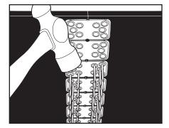
**19**. Remove MBRTA. Remove pilot nails and clips with a hammer. If fasteners are 1" (25mm) or more from edge of belt, notch belt. Remove nails from MBRTA.
