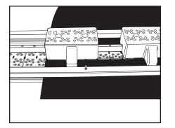
**16**. If all plates are not covered by guide blocks (E), move a guide block (E) to install remaining rivets.
