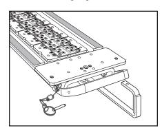
**5**. Insert cam rods (C) through holes in clips across bottom of tool.
