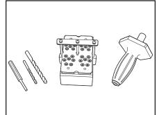
**NOTE**: MBRTA cannot be used to install single or double-plate BR-10 or BR-14 fasteners. Refer to RSP310.
