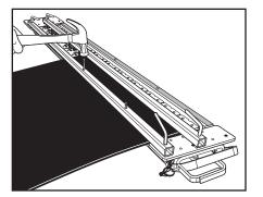
**11**. Secure belt by driving double headed nails through holes in clamp bar and into the belt.
