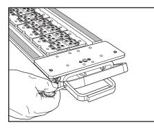
**6**. Turn cam rods (C) to lock fasteners in place. Secure cam rods (C) to channel base handle (D) with pin.
