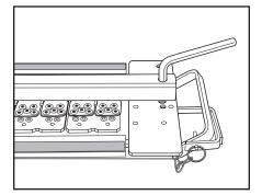
**9**. Attach clamp bar (B) to the tool so that one edge of the clamp bar is over the center of the fastener strips. Tighten clamp bar.
