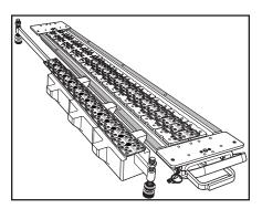
7. Turn over aligning bar (A) and align guide blocks with bottom plates. Place top plates on guide blocks, Flexco<sup>\*</sup> facing up.
