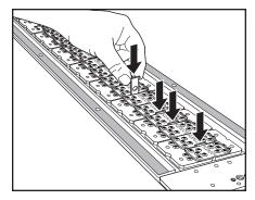
**4**. Insert a clip between first and second plates at each end of the fastener strips. Insert clips on both sides of center plate of each fastener strip.
