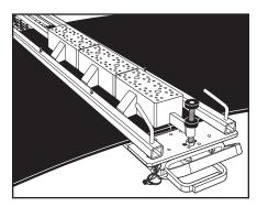
**13**. Insert aligning bar in ends of MBRTA. Tighten top knurled nut. Tighten lower knurled nut to lower fasteners to belt surface.
