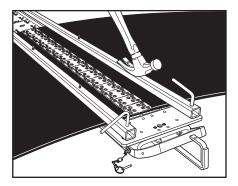
**18**. Unlock and remove cam rods (C). Remove nails and clamp bars (B).
