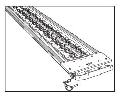
**3**. Starting at the right side of the tool, place proper number of fasteners on anvil plates (F) with Flexco<sup>\*</sup> facing up.
