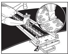
17. For easier troughing on belts up to 35° trough, remove bridges between plates in troughing area using the BR151 Bridge Removal Tool.
