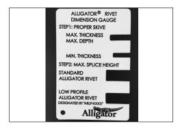
Alligator® Rivet fasteners require proper skived belt thickness, fastener clinch, and rivet curl. The enclosed Alligator Rivet Dimension Gauge is provided to ensure proper installation.
