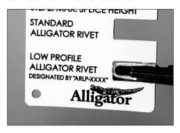
**4.** Measure finished splice height to ensure fastener has been properly installed. Based on the fastener you installed (standard profile or low profile), insert installed splice into the appropriate slot. The gauge should slide over each plate in the fastener strip. If the gauge does not slide easily over, reinsert in tool and install further.
