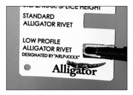
**4.** Measure finished splice height to ensure fastener has been properly installed. Based on the fastener you installed (standard profile or low profile), insert installed splice into the appropriate slot. The gauge should slide over each plate in the fastener strip. If the gauge does not slide easily over, reinsert in tool and install further.
