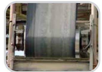
*Ensures centre loading by installing before the tail pulley.*
