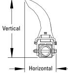
**Horizontal Clearance Required** 175 mm **Vertical Clearance Required** 475 mm
