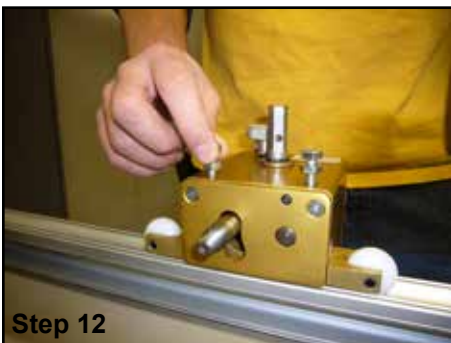
Step 12: Finger tighten top and bottom adjusting bolts.
