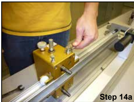
Step 14: Tighten the top and bottom lock nuts.
