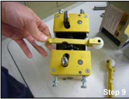
Step 9: If clevis bracket guide roller assemblies were removed, reinstall with the notch in the clevis bracket positioned over and facing the roller shaft.
