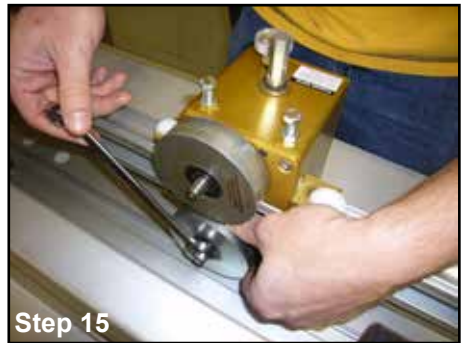
Step 15: Reinstall rollers. While turning the roller, tighten the nut until the roller just starts to rub against the extrusion. Now back nut off about ¼ to ½ turn.
