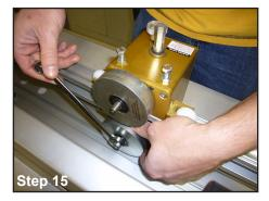
**Step 15:** Reinstall rollers. While turning the roller, tighten the nut until the roller just starts to rub against the extrusion. Now back nut off about  $\frac{1}{4}$  to  $\frac{1}{2}$  turn.
