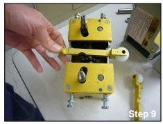
**Step 9:** If clevis bracket guide roller assemblies were removed, reinstall with the notch in the clevis bracket positioned over and facing the roller shaft.
