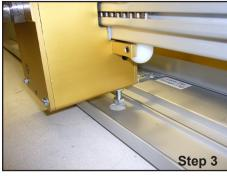
Step 3: Position the head over the access holes in the bottom pan.
