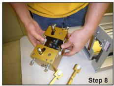
Step 8: Install the four stabilizing wear clips in position.
