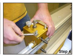
Step 4: Break loose all four jam nuts (top and bottom of head).
