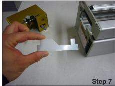
Step 6: Remove head from extrusion. Step 7: If your lacer is equipped with the stabilizing wear strip, remove and discard it.
