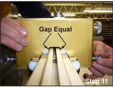
**Step 11:** Adjust the top bolts so that the gap between head and extrusion is equal.
