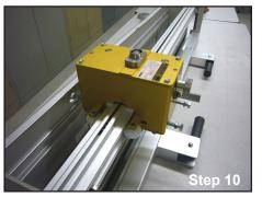
**Step 10:** Place head back on extrusion, positioning it so bottom adjusting bolts are over the access holes in bottom pan.
