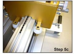
Step 5: Loosen top and bottom adjusting bolts until guide rollers clear extrusion channel (Step 5a - 5c).
