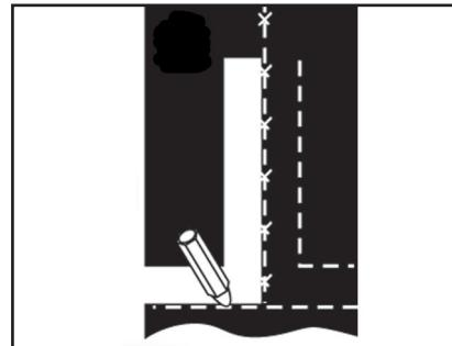
2. Square belt using centerline method. Cut belt using a Flexco belt cutting tool.
