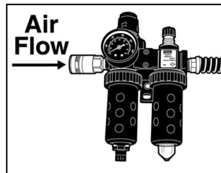
3. Hookup your air compressor to the "in" side of the regulator kit with a 3/8" fitting. Use compressed air directly from an air compressor. **WARNING: Do not use any bottled gases, including oxygen, to operate this tool. Explosion will occur.** Air pressure should maintain 8 SCFM at 75 PSI through the 3/8" fitting. The regulator is factory preset at 75 PSI and is not adjustable. **CAUTION: Increasing PSI beyond 75 PSI will damage the tool.**
