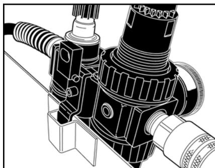
2. Mount regulator kit on the tool box. Insert hook on the back of the regulator kit into the slot on the tool box. The regulator kit must remain level during tool operation. Fill oiler with SAE #10 non-detergent oil. **CAUTION: Do not substitute SAE #10 oil with other types of lubricants, the power driver will not function and will be permanently damaged.**
