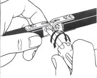
Use finger to keep rocker pin centered in fastener. Turn pin with screwdriver until you feel a slight click.
