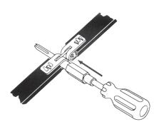
Push rocker pin into fastener (don't force)—turn screwdriver while applying slight pressure.
