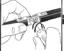
Use finger to keep rocker pin centered in fastener. Turn pin with screwdriver until you feel a slight click.
