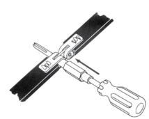
Push rocker pin into fastener (don't force)—turn screwdriver while applying slight pressure.
