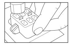
3. Push male or female half of fastener over belt and into recess in holder as far as it will go. Look into staple slot in holder and make sure holes in fastener are visible. Drive staple into belt flush with holder.
