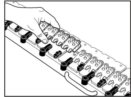
3. Lift and turn gauge pin guides to R2/R5/R5½ setting. Center fastener strips on MSRT or SRТА application tool.
