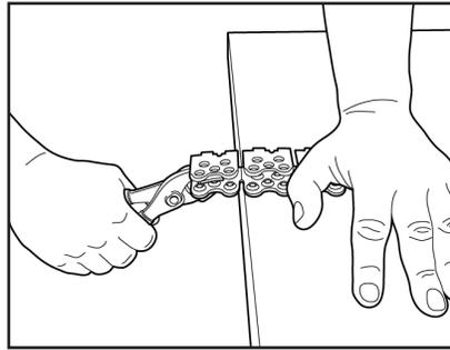
2. If a shorter fastener strip is needed, break off extra plates by bending strip at the checkpoints with pliers. Do not use single plates.
