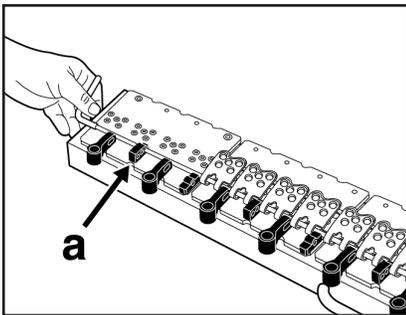
4. Insert gauge pin through (a) guides and fastener loops.
