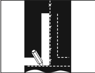
1. Square belt using centerline method. Cut belt 4" (100 mm) behind old splice using a Flexco belt cutting tool. Skive belt when top cover permits.
