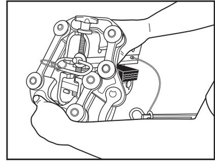
3. Slide scissors onto the clamp bar. Place top of scissors over the pre-clamping screw and then slide the bottom of the scissors over the bottom of the clamp bar. Repeat on the other side.
