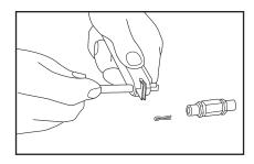
**6.** When ready to join ends remove both cotter pins. (1 cotter pin in each half fastener.) Discard cotter pins. To remove assembly clip, use the rocker pin tool. Give rocker pin one-half turn, then push out.
