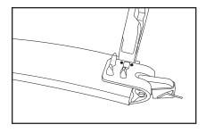
**4.** Start clinching of nails with slotted end of alignment pin, then complete with pliers. Do not crush fastener. Repeat above operations on opposite end of belt using unit with assembly clip.
