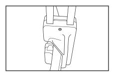
1. Square belt end with Alligator\* V-belt cutter. Read "Belt Length" guidelines on reverse side before cutting belt to correct length.
