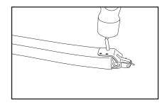
**3.** Fit assembled unit with links on one end of belt. Place on soft wood block. Drive nails through fastener and belt into soft wood block. Be careful not to distort belt by pounding fastener.
