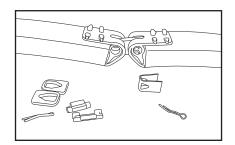
**7.** Fastener ready for assembly. Note aligning pin, two piece rocker pin, and flat-sided hole in link which fits into seat in rocker pin.
