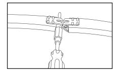
**8.** Assemble rocker in tool, rocker pin and aligning pin in sleeve as shown. Then push through fastener and twist. Rocker pin will push out alignment pin. Turn rocker pin until seat locks into position in link.
