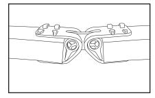
9. Important—Make sure both rocker pins are locked into link in the correct position. The screwdriver slot in the large section must be parallel with the length of belt and away from the belt as shown. When centered and in this position, the rocker pin locks automatically.
