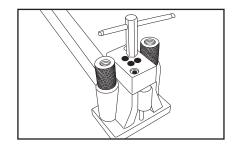
2. Clamp belt against Stop in Piercing Tool. Drive the punch into shoulder and STOP. Repeat for each hole. The punch never goes all the way through the belt.
