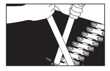
**12.** Break off excess bolt ends using two bolt breakers. Peen or grind bolts to finish.
