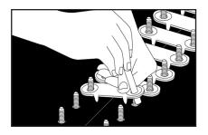
**6.** Place top plates over bolts using bolt horn.
