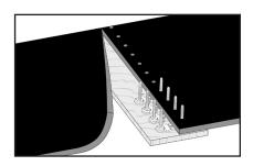
**4.** Fold one belt end back and insert bolts in one row of holes.
