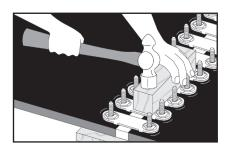
**11.** Hammer plates in belt with wood block. Retighten nuts.
