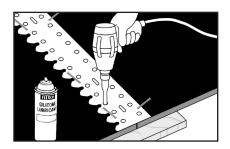
NOTE: A ½" square drive electric impact wrench with Flexco 5552 Quick Change Chuck will speed hole boring operation. Max torque: 250 Lb-Ft (340 N-m).
