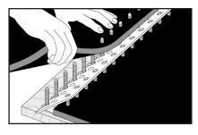
**5.** Align bolts with templet teeth and place the other belt end over bolts. Remove templet.
