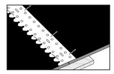
**2.** Support belt ends with wood plank. Nail Flexco Templet in position with belt ends tight against lugs.
