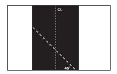
**NOTE:** For a 45° Splice, cut squared belt end on a 45° angle. Use the 45° cut belt end as a guide for cutting off the other end of the belt. Make sure that center lines match up and are straight.
