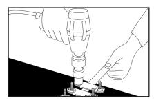
**9.** Pull tape tight and hold in position by tightening a fastener at each end. Then tighten all other plates.
