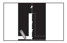
1. Square belt ends using centerline method. Cut belt ends using Flexco 900 Series Belt Cutter.
