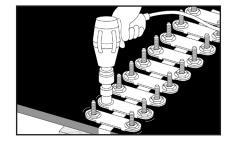
10. Tighten all fasteners from edges to center. Tighten all nuts uniformly. NOTE: A Flexco Power Wrench used with an impact tool will speed this step considerably.
