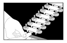
**8.** Cut Flexco-Lok® Tape 3-1/2 times the belt width and feed tape under top plates, under the bottom plates, then back under top plates.
