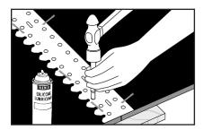
**3.** Spray templet holes with Flexco Silicone Lubricant. Punch or bore bolt holes. Remove templet.
