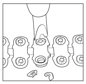
1. Place Cracking Chisel over the nut and hit with a firm blow. Use a 2 lb. or heavier hammer. Be sure to wear safety goggles. **NOTE:** Position worn plate over solid backing before striking chisel.
