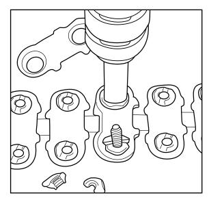
After nuts are removed, replace plates, bolts, and nuts.
