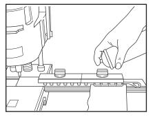
**7.** With the comb assembly to one side, spray a light covering of Alligator Plastic Rivet Lube (PRL4) on the rivet ends.
