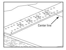
2. Place templet over belt end, aligning centerlines and, make sure belt end is tight against templet lugs. Slide second belt end under templet, against lugs. Align centerlines. Nail or clamp the templet in place. Drive nail halfway into belt and bend nail over.
