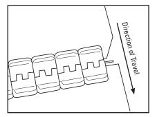
**11.** Mesh the two belt ends together and insert the hinge pin. Notch the trailing belt end, and, using pliers, bend the end of the pin to prevent migration.
