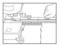
**10. Installing fasteners on a wide belt:** Insert the other side of the belt end in the comb. Insert the gauge pin, tighten the clamp screws, and continue as before.
