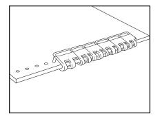
**4.** Install the fasteners across the belt by opening each plate enough to slide it over the belt. Insert the rivets from the top placing the smooth side of the fasteners on the top side of the belt. Squeeze each plate to make certain that it is inserted fully.
