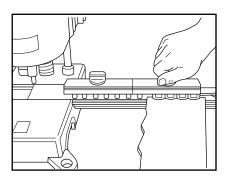
**9.** Remove the gauge pin, loosen the clamp screws, and remove the belt from the comb assembly. Repeat the procedure on the second belt end.
