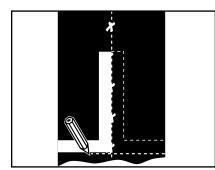
1. Square belt end at right angle to center line. Cut belt using a Flexco belt cutting tool.
