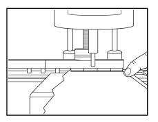
**8.** Turn on the tool. Line up an end rivet with the curling bit and apply pressure to the rivet. Make certain the curling bit contacts the rivet end only. Maintain pressure until the rivet is formed into a tight, low profile curl.
