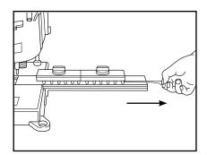
6. Slide the comb assembly to one side and remove the gauge pin. Insert one end of the belt into the comb. Insert the gauge pin and tighten the clamp screws by hand until the fasteners are pressed firmly against the belt surface.
