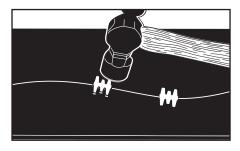
**3.** Drive fastener teeth into the belt and supporting board with a hammer. Avoid hitting the center of the plate.
