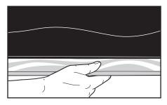
1. Place a wood support under belt where rip is to be repaired. Do not install Turtle\* fasteners using the conveyor pulley or other metal surface as support, as fastener teeth would not be properly cinched.
