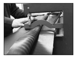
3. With the edge of the bottom cover against the belt stop, fold back the top cover and clamp.
