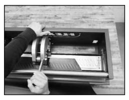
20. Punch belt and cut away excess. NOTE: Be sure none of the top cover fingers are out of alignment underneath the punch block throughout punch process.
