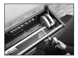
11. Unclamp the belt clamp and move the belt to the left, align fingers to the punch board blades confirming the distance from the leading edge of the belt end to the belt stop is correct.
