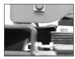
**13.** (**Belt End 2**) Position the leading belt edge up against the belt stop, aligning the right edge up with the valley of one of the punch board cutting blades on the right side of the PUN M<sup>™</sup>. Fold the bottom cover under and clamp between the clamp bar.
