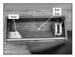
2. (Belt End 1) Position the leading belt edge up against the belt stop, aligning the left edge up with the peak of one of the punch board cutting blades.
