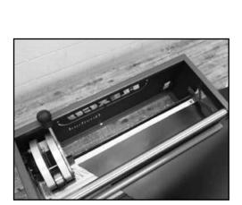
**8.** Unlock the belt tray clamps and slide the tray to the forward position.
