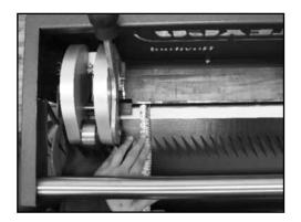
**21.** Unclamp the belt clamp and move the belt to the right, align fingers to the punch board blades confirming the distance from the leading edge of the belt end to the belt stop is correct.
