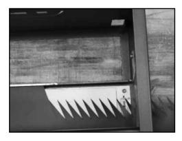
15. Unclamp the clamp bar and shift belt to the right. Align punched fingers with cutting blades on right side of punch board making sure leading belt edge is tight up against the belt stop. Re-clamp belt.
