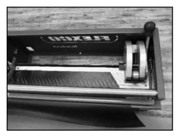
**18.** Unlock the belt tray clamps and slide the tray to the forward position.
