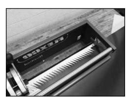
9. Punch belt and cut away excess. NOTE: Be sure none of the fingers are out of alignment underneath top cover prior to resuming punch process.
