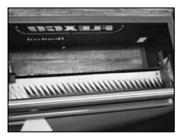
**16.** Repeat process until the entire width of belt has been punched then remove belt.
