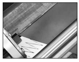
7. Unclamp the belt, remove and then re-insert the belt into the PUN  $M^{\text{\tiny M}}$  with the leading edge of the top cover up against the belt stop and the left edge aligned with the peak of one of the punch board blades, then clamp.
