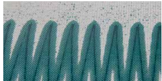
Excessive bleed through
