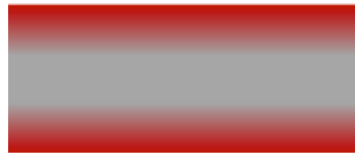
Example of heat not fully penetrating belt thickness
