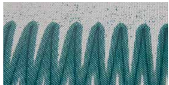
Excessive bleed through
