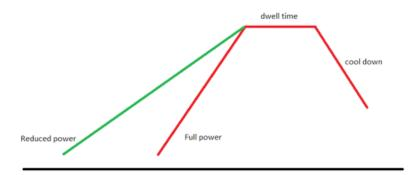
Depending on power used, the press might operate in 'full power' mode, which will have a quicker warm up time, or in the 'reduced power' mode. 'Reduced power' mode will take slightly longer to reach the desired dwell temperature. Actual dwell time and cool down will take the same amount of time in either power mode.
