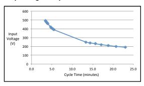
In this instance, the likely culprit is the difference between the 480V and 230V power source, but there are actually a number of factors that should be considered. Here are a few things to think about when voltage variances could be a factor in the length of time to complete a splice:
