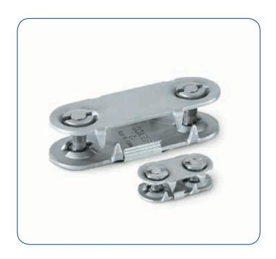
belt's top cover with a router to a depth of about 4.8 mm (3/16") so the top plates would nest flush with the surface. Finally, top and bottom plates were drawn tightly into the belt with two heat-treated bolts, while short teeth formed into the plate edges near the bolts increased each plate's grip. These special bolts, inserted upwards from the underside of the belt, have flat heads that seat into pockets formed in the bottom plates to assure smooth passage across drive pulleys and idlers.
