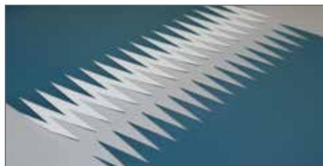
The FOF splice is created by separating the plies and punching fingers on the two layers on an overlap. This allows for two linear bonds in addition to the bond between the offset layers. Typical FOF splices will be at least 25% stronger than standard FS of the same belt material.
