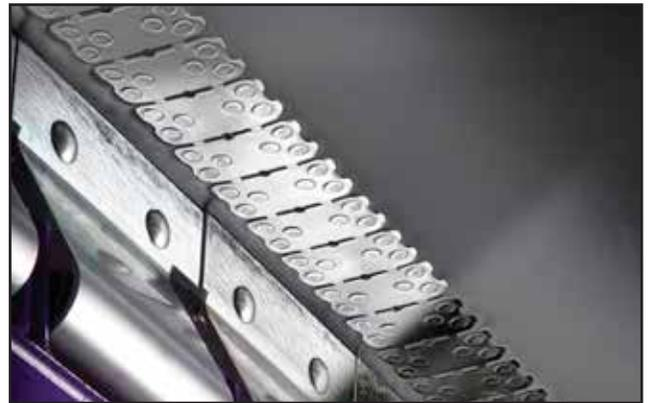
top cover of a belt is greater than 3/16", skiving is always recommended. Skiving does not affect the strength of the belt or the splice because only the top cover is removed, which does not affect the carcass. Deeper penetration of the fastener teeth into the belt carcass can also reduce return idler noise, minimize wear on idler bearings, and eliminate impact with skirting material.
