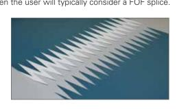
The FOF splice is created by separating the plies and punching fingers on the two layers on an overlap. This allows for two linear bonds in addition to the bond between the offset layers. Typical FOF splices will be at least 25% stronger than standard FS of the same belt material.
