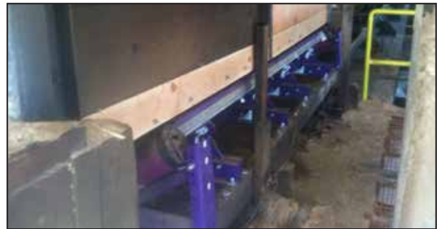
To seal the load zone properly, the clamping mechanism should be both durable and provide a strong hold. Paired with a belt support system that provides an even and consistent surface, a proper seal is achieved.
