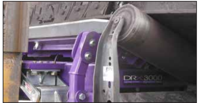
In some cases impact idlers are enough, while others may need a true impact bed to provide the required protection for the belt.
