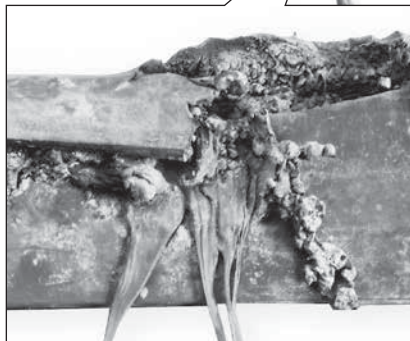
Urethane blade damage from friction and thermal changes
