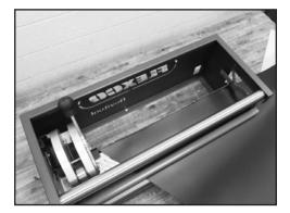
7. Unclamp the belt, remove and then re-insert the belt into the PUN M<sup>™</sup> with the leading edge of the top cover up against the belt stop and the left edge aligned with the peak of one of the punch board blades, then clamp.
