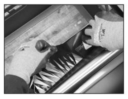
**4.** Begin punching bottom cover by following instructions beginning on pg.33 of the **PUN M<sup>™</sup> Manual Finger Punch Safety and Operation Manual** until you've utilized the complete cutting surface of the punch board, then cut off excess.
