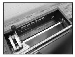
**8.** Unlock the belt tray clamps and slide the tray to the forward position.
