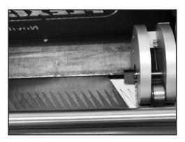
17. Unclamp the belt, remove and then re-insert the belt into the PUN M<sup>™</sup> with the leading edge of the bottom cover up against the belt stop and the right edge aligned with the valley of one of the punch board blades, then clamp.
