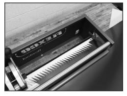
9. Punch belt and cut away excess. NOTE: Be sure none of the fingers are out of alignment underneath top cover prior to resuming punch process.
