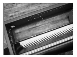
14. Begin punching top cover by following instructions beginning on pg.37 of the PUN M<sup>™</sup> Manual Finger Punch Safety and Operation Manual until you've utilized the complete cutting surface of the punch board, then cut off excess.
