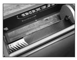
**5.** Unclamp the clamp bar and shift belt to the left. Align punched fingers with cutting blades again on left side of punch board making sure leading belt edge is tight up against the belt stop. Reclamp belt.
