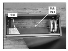
**2.** (Belt End 1) Position the leading belt edge up against the belt stop, aligning the left edge up with the peak of one of the punch board cutting blades.
