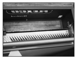
**16.** Repeat process until the entire width of belt has been punched then remove belt.
