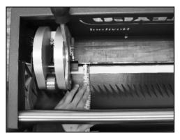
**21.** Unclamp the belt clamp and move the belt to the right, align fingers to the punch board blades confirming the distance from the leading edge of the belt end to the belt stop is correct.
