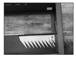
**15.** Unclamp the clamp bar and shift belt to the right. Align punched fingers with cutting blades on right side of punch board making sure leading belt edge is tight up against the belt stop. Re-clamp belt.
