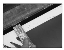
**10.** Prior to releasing the clamp bar and repositioning belt to the left, measure the distance from the leading edge of the belt end to the belt stop and record the measurement.
