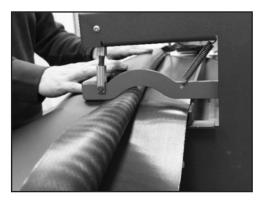
3. With the edge of the bottom cover against the belt stop, fold back the top cover and clamp.
