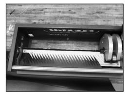
**20.** Punch belt and cut away excess. **NOTE: Be sure none of the top cover fingers are out of alignment underneath the punch block throughout punch process.**
