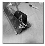
**3.** Slide the replacement spring onto the adapter as shown. Remove the screwdriver once it touches the adapter.
